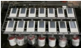
Binary lead alloys on a test rack at TNO in Den Helder.
